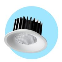
Ø105mm x H56mm (Cutout: Ø92mm) 10W • 853lm (at 3000K) • 60° Beam LED Lifetime: >59.000h L70B10 Colour Deviation: SDCM≤3
